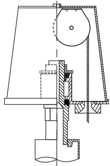
**Revolving Internal Halyard Truck**
